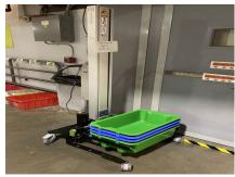
1 photo of a Lift'N Buddy power hand truck used to transport, raise and lower totes with and without material inside. This equipment has a smaller foot print than the tote lifters.
